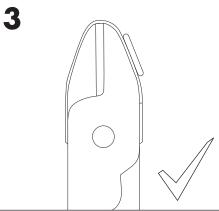
**Important:** Turn instrument and check that there is no gap between Catch-Tray and Snippers+.
