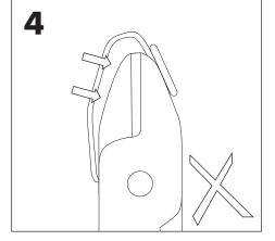
Attach Catch-Tray from the left side then turn 90° in the instrument axis.
